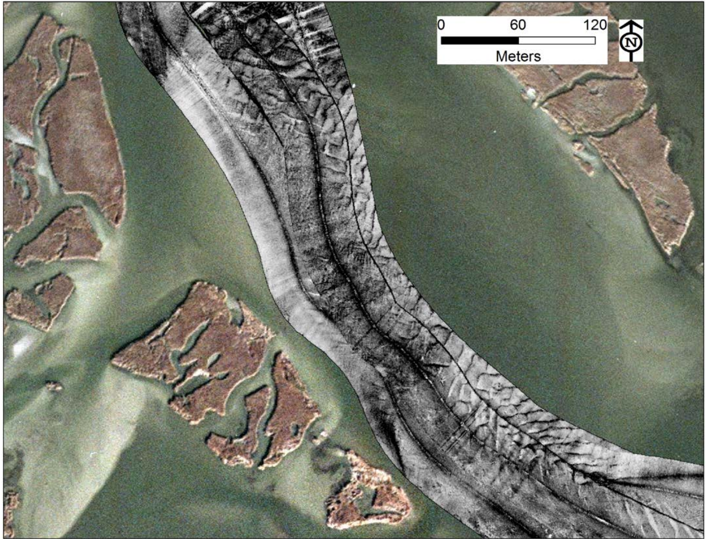
Figure 2. An example of seabed features identified in the sidescan sonar mosaic at the entrance to Lynnhaven Bay. Large sand waves are indicative of a dynamic and high tidal energy environment.
